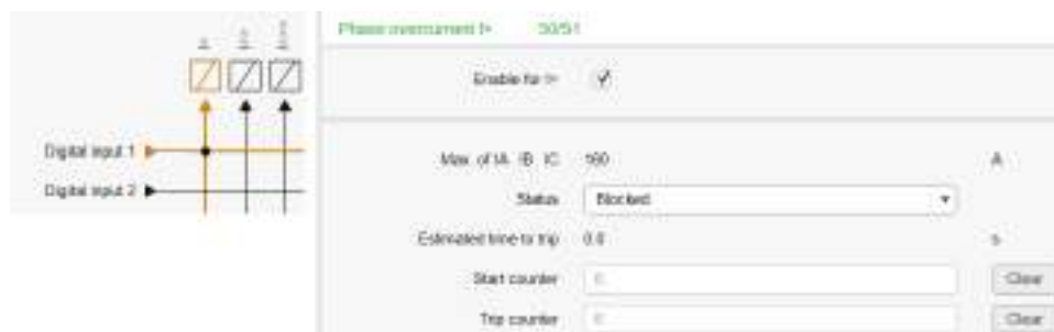
Figure 344 - A view from the setting tool showing a DI input blocking connection (left picture) and the result for the I> stage when the DI is active and the stage exceeds its current start value
