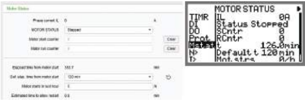
Figure 81 - Motor status via eSetup Easergy Pro and local panel
