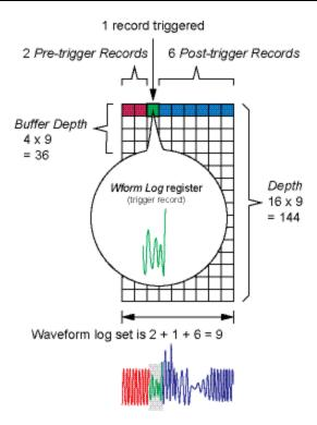
The waveform log set for the extended waveform capture = [pre-trigger records] + [actual trigger record] + [post-trigger records]. The total waveform records captured in this example is 2 + 1 + 6 = 9.
