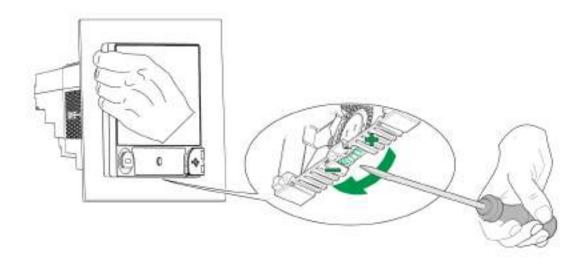
2. Carefully pull the display away, far enough to access the cable connector on the display.
