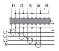
For a 3-phase 4-wire system, the meter measures the residual current for Ground at I5.
