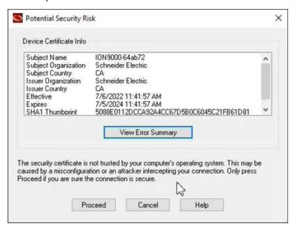
ION Setup stores the certificate when using Network mode. In Single Device mode, you must accept the certificate every time you connect to a device using Secure ION.
