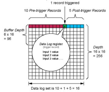
Burst data log set = [pre-trigger records] + [post-trigger records] + [actual trigger record] = 10 + 5 + 1 = 16.
