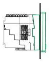
Holding the display, turn the tightening wheel with a flat-head screwdriver until it disengages from the display.
