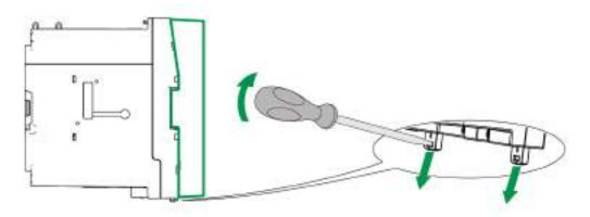
2. Holding the meter firmly, swing it outwards and pull slightly upwards to detach it from the top retaining hooks.
