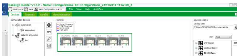
Figure 94 – Configuring local acquisition for Saitel DP
