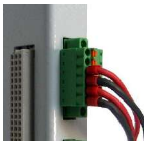
Figure 51 – Connecting external power supplies to a SM_BPX
