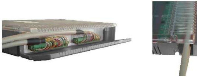
Figure 73 - Position of the cables when they are installed
