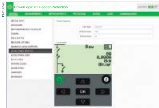
PowerLogic P3 web-HMI
